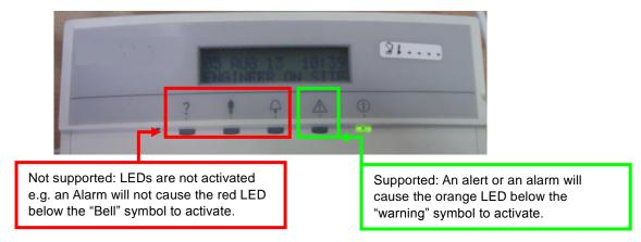
*Note:* For migration, alarm indication on the Sintony keypad is now announced by the flashing of an orange LED below the "warning" symbol.
