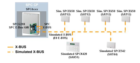
Note: Simulated X-BUS = Physical E-Bus which has been simulated and appears to the SPC controller as X-BUS
